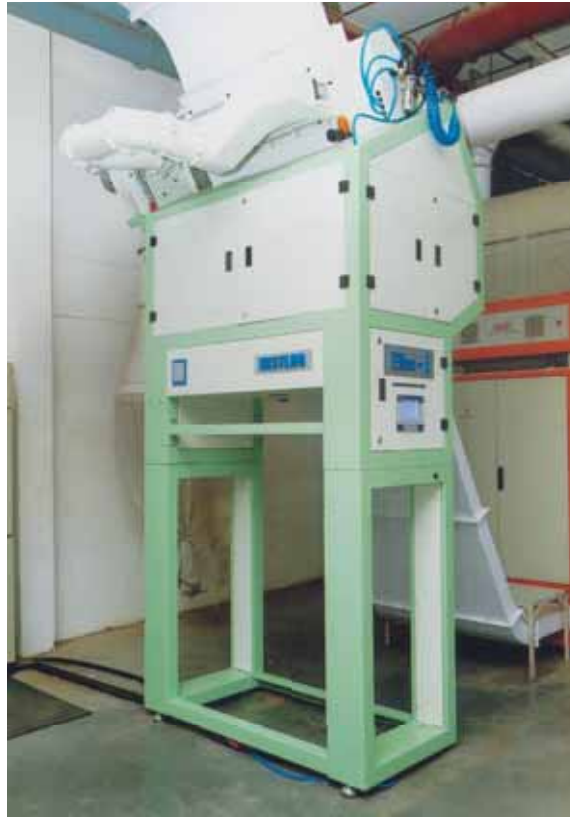
A view of the "Nestling Blue-i" scan contamination removing machine installed in our Unit – II Blowroom at Rajapalayam.
